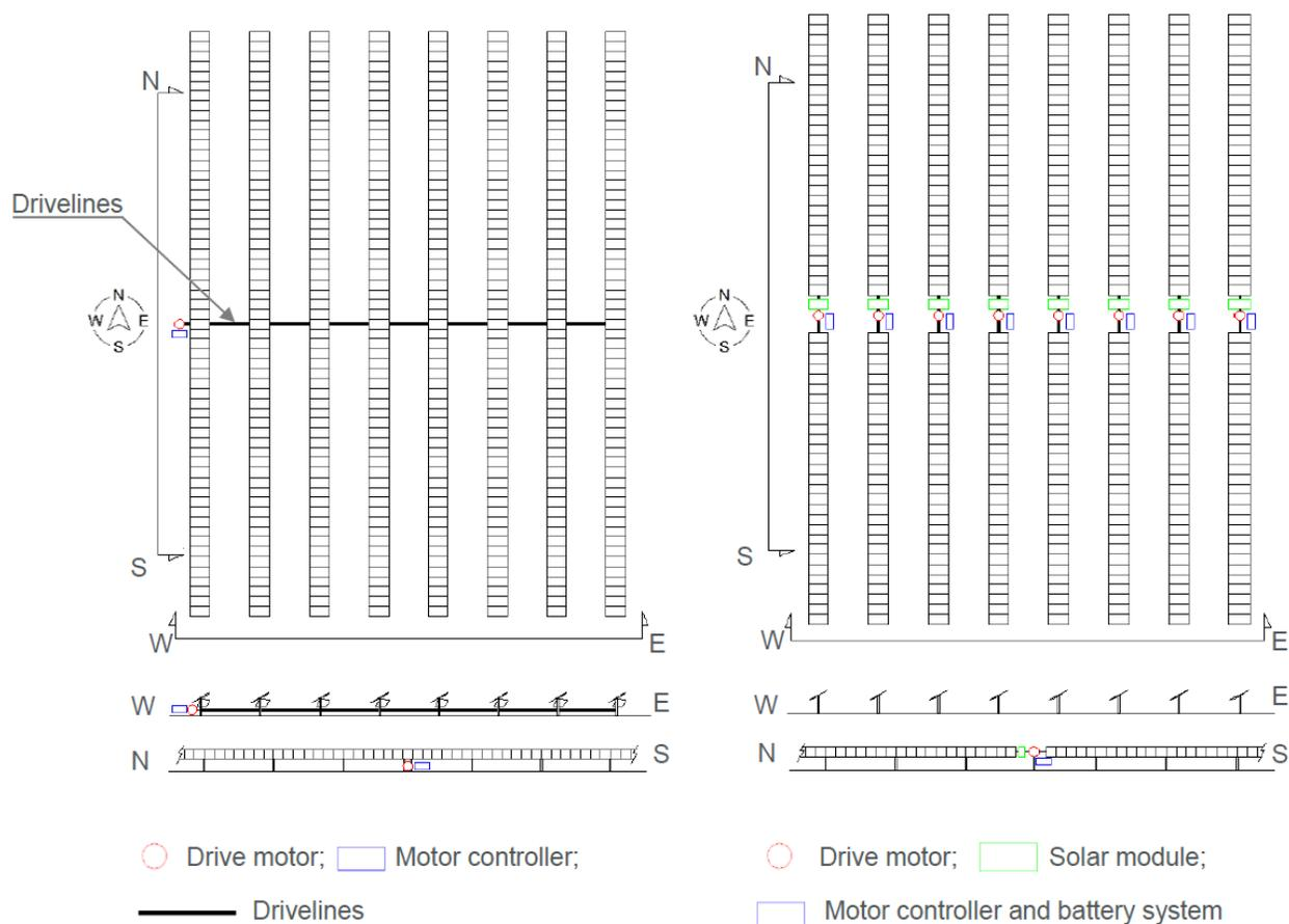
**Figure 53. Multi-row (left) and single-row (right) tracking systems.**
