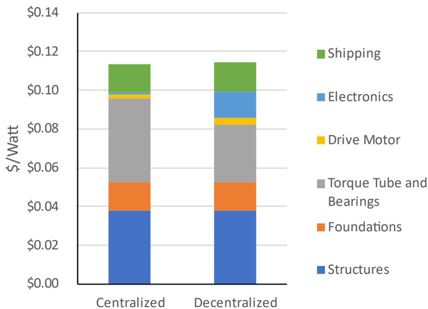
**Figure 54. Indicative cost breakdown of trackers, by subcomponent.**
