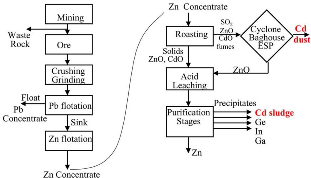
Figure 69. Cd flows in Zn mining and refining.
