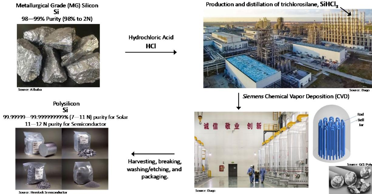
**Figure 23. Steps to produce polysilicon from MGS, Siemens chemical vapor deposition method.**
