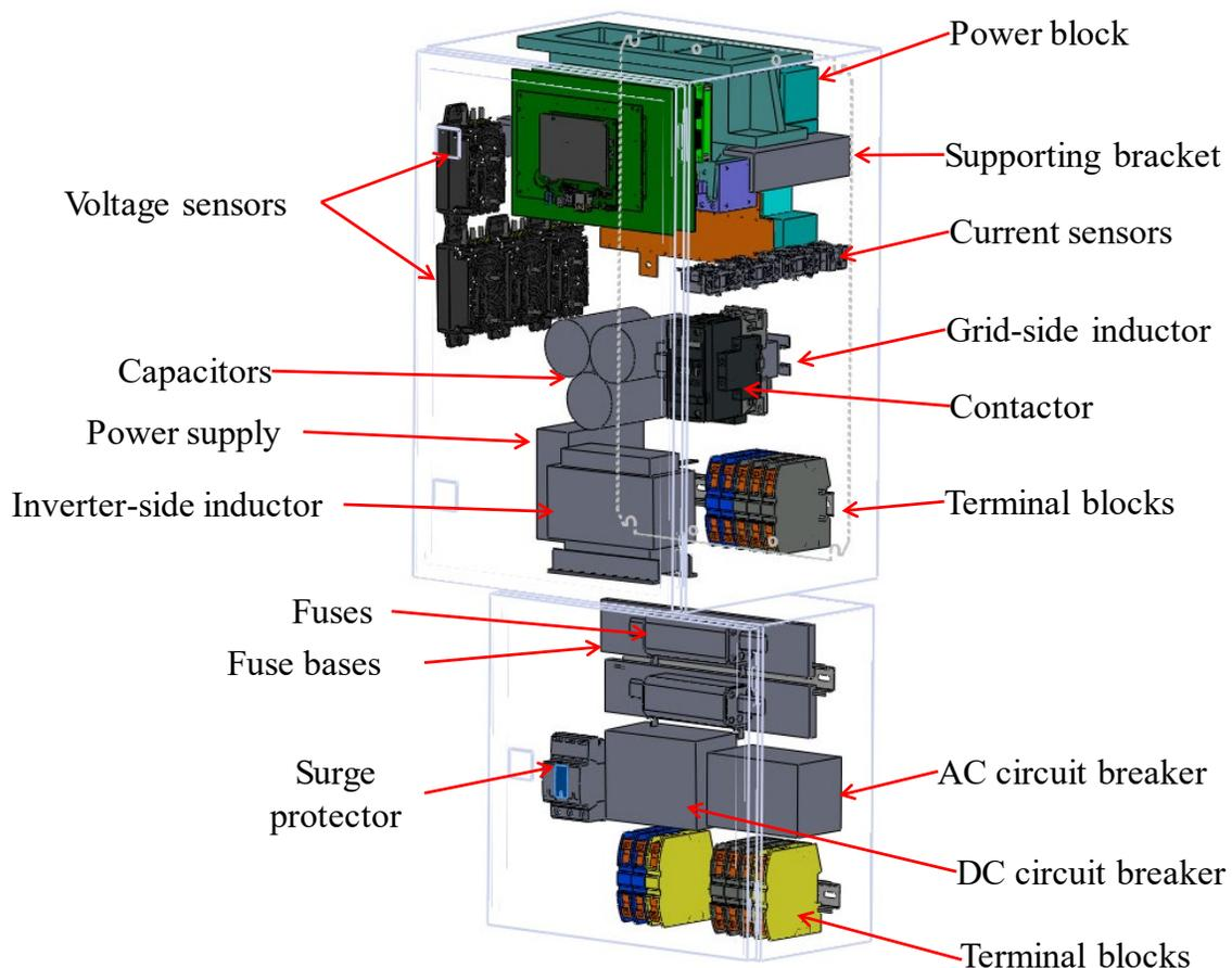
**Figure 59. Inverter assembly with supporting components.**
