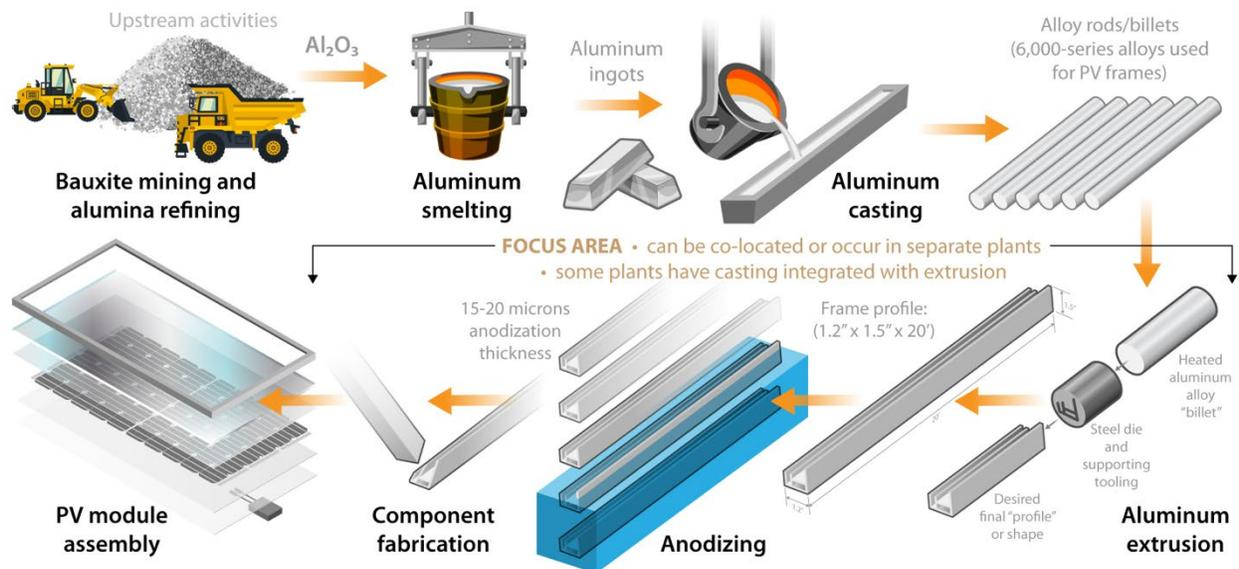
**Figure 21. Production process for aluminum module frames, assuming primary aluminum extraction.**
