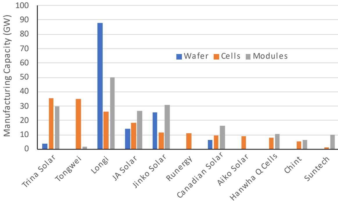
**Figure 43. Wafer, cell, and module manufacturing capacities of some leading cell and module manufacturers.**
