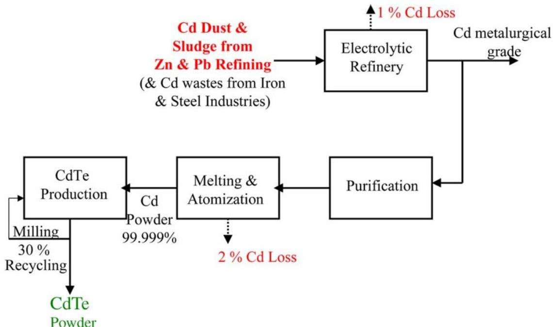
**Figure 70. High purity CdTe production flow.**
