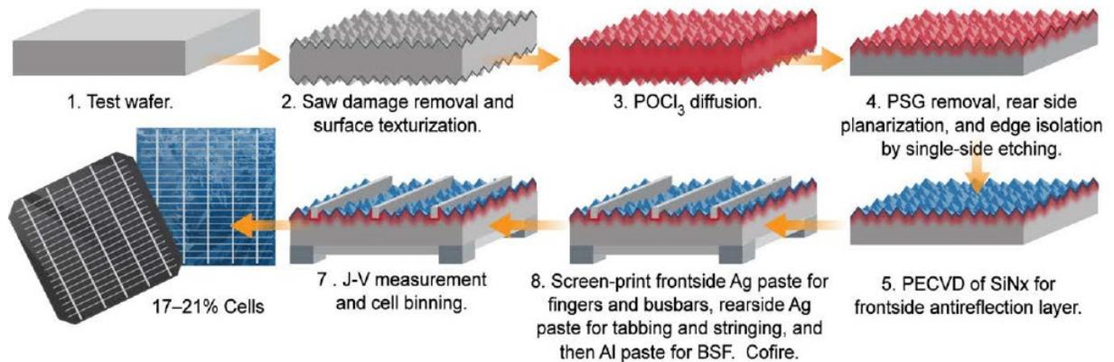
Figure 36. Process flow for manufacturing standard full-area Al-BSF cells.
