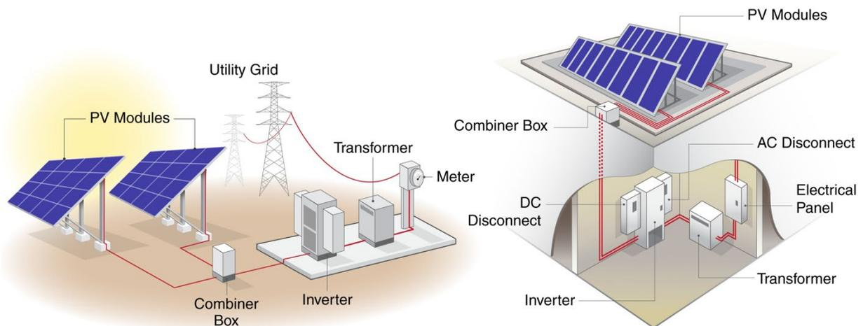
**Figure 1. Illustrations of a utility-scale PV system (left) and a commercial rooftop system (right).**
