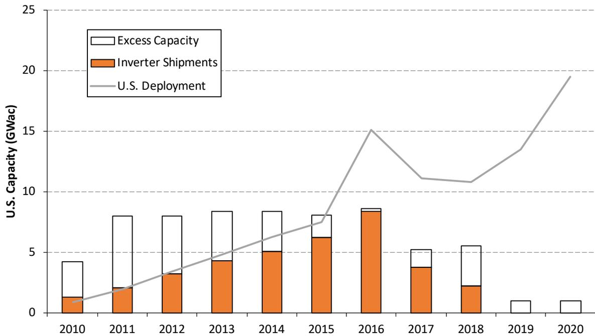
**Figure 66. U.S. inverter production, manufacturing capacity, and system deployment.<sup>4</sup>**
