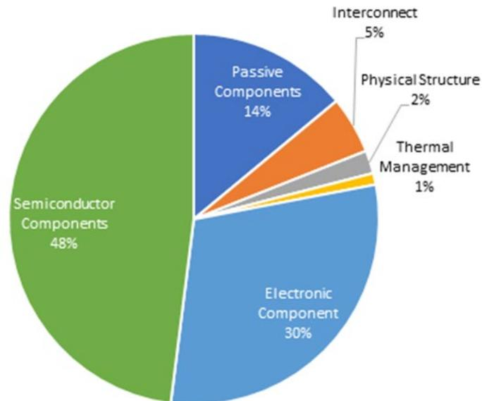
**Figure 60. Breakdown of silicon carbide inverter material costs.**
