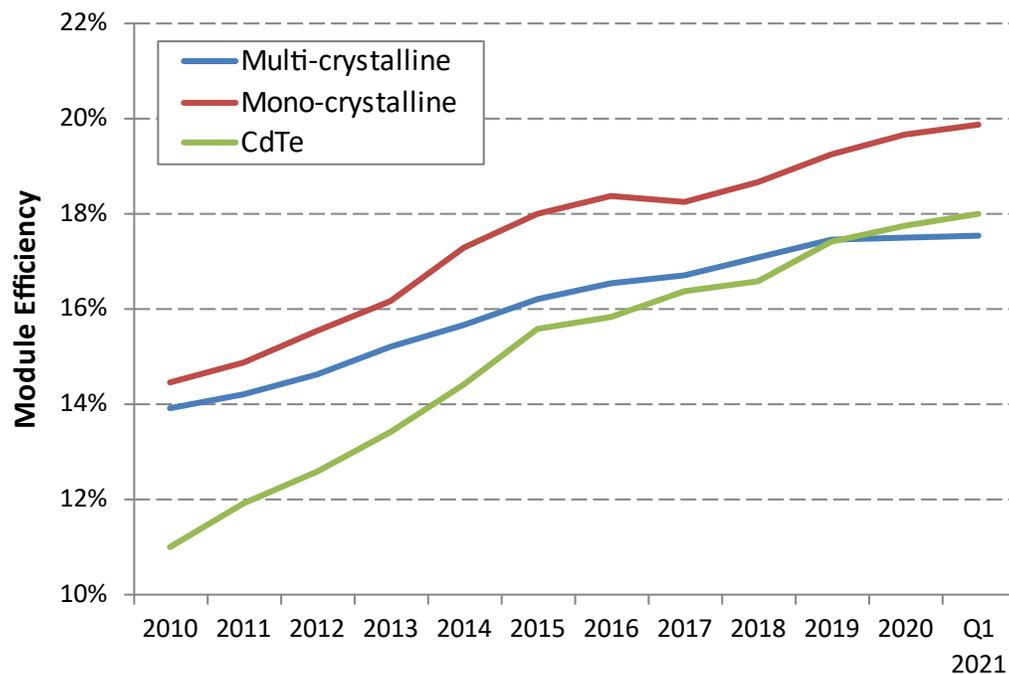
**Figure 75. Efficiencies of c-Si and CdTe modules.**
