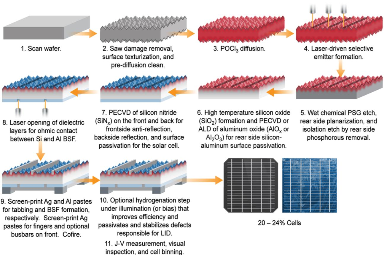
Figure 37. Process flow for manufacturing standard full-area PERC cells.
