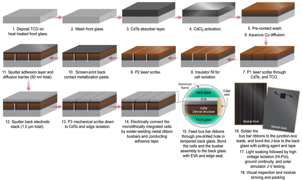
Figure 73. Process flow for making CdTe modules.
