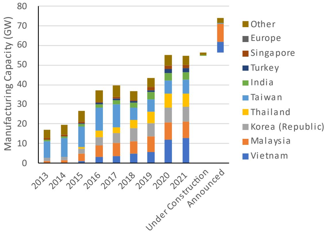
**Figure 41. Cell manufacturing capacity outside of China.**
