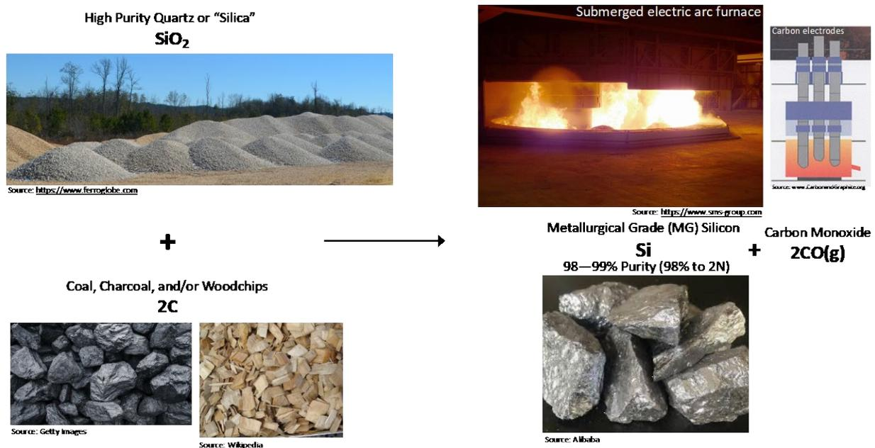
Figure 13. Principal input materials and process for MGS production.
