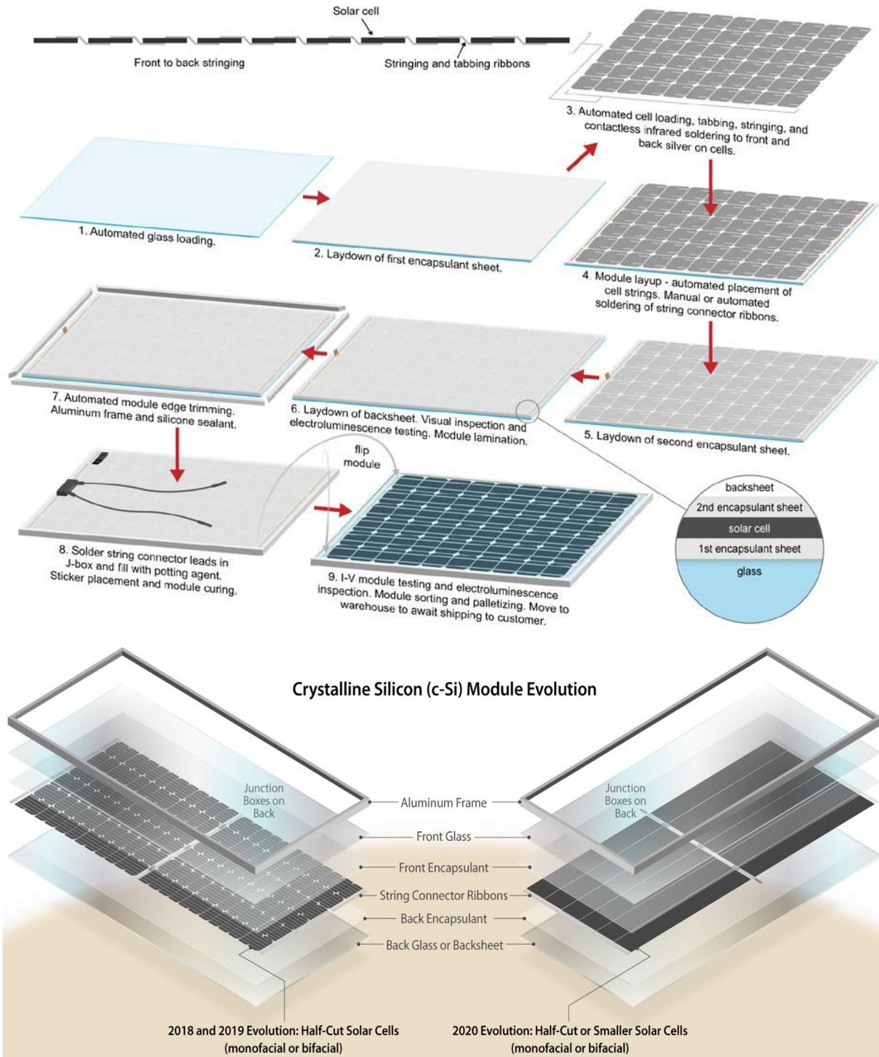
Figure 45. Process flow (top) and finished product (bottom) for standard 60-cell monocrystalline-silicon module assembly.
