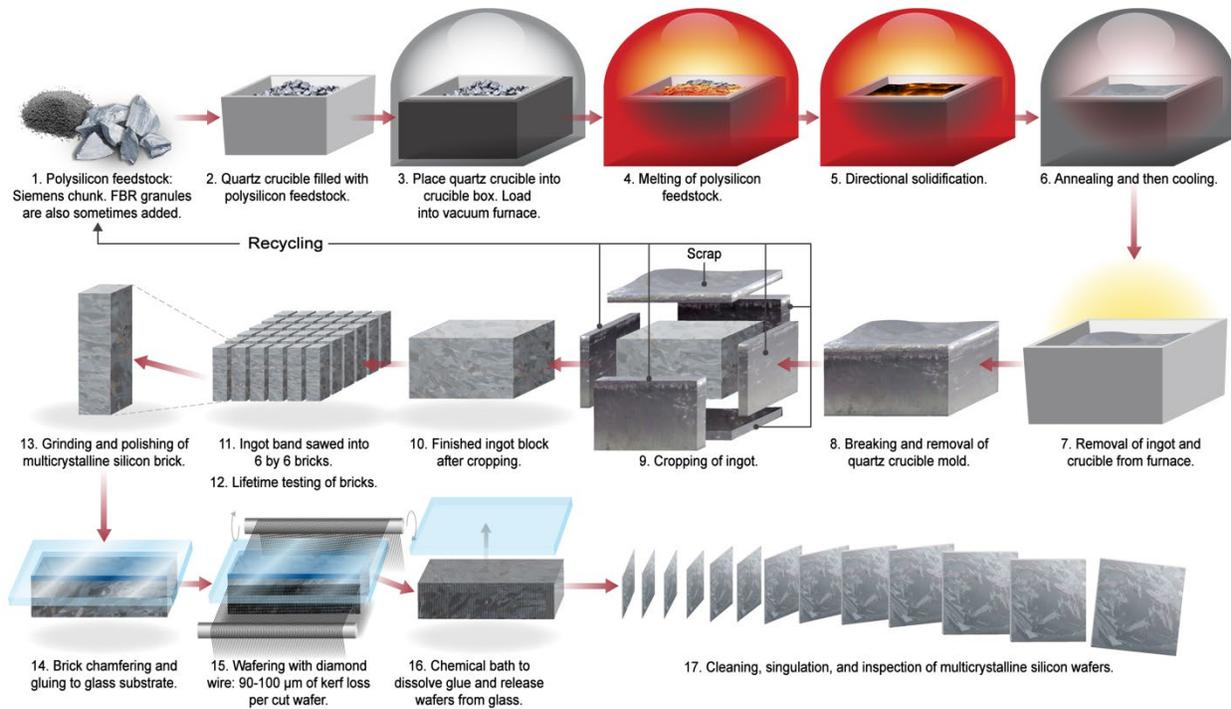
**Figure 30. Process flow for making multicrystalline-silicon wafers via directional solidification (DS).**
