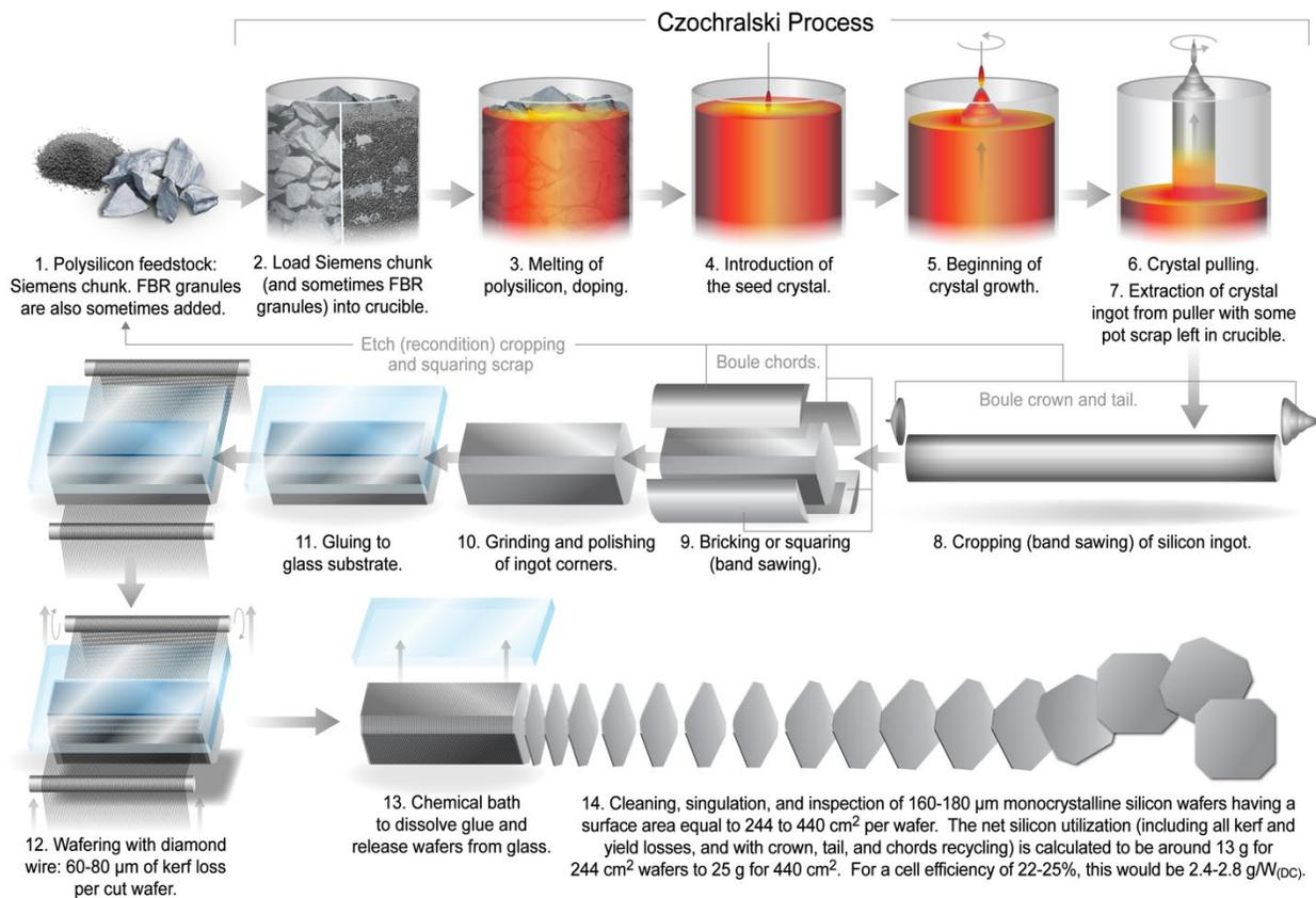
**Figure 29. Process flow for making monocrystalline-silicon wafers via Cz crystal growth.**
